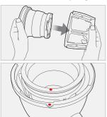
Place the juicing screw into the strainer. Turn and press down on it until it clicks into place.
